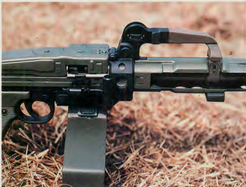
ABOVE: MG82 has durable, hard-baked, olive-drab finish. LEFT: Unlike MG42, 82 is entirely recoil-operated, not gas-assisted. BELOW: Quick-change barrel allows three-second barrel change. RIGHT: MG82 trigger-group assembly is identical to MG42. Receiver is stamped with serial number 10.
